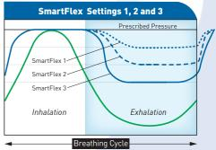
SmartFlex offers three pressure reduction settings that will automatically reduce the pressure generated by the IntelliPAP upon exhalation and raise the pressure back up to prescribed pressure at the onset of inspiration. The settings correlate to an exact cm  $H_0$  D ressure drop – so a setting of 1 = 1 cm  $H_0$ D drop in pressure during exhalation.
